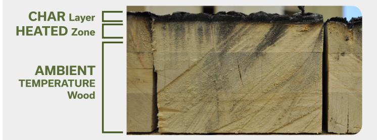
**Case in Point:** A successful ASTM E119 fire endurance test of a cross-laminated timber wall was key to the decision to recognize CLT in the 2015 edition of the IBC<sup>®</sup>. While only seeking a two-hour rating as required by building code provisions, the test specimen lasted three hours and six minutes.\*
