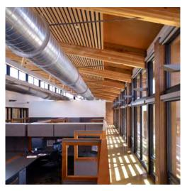
Inverted king-post trusses with laminated wood beams offer a high strength-to-weight ratio and exceptional ductility for improved structural performance during times of strong desert winds or seismic events.
