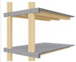
Hybrid floor slab and double wood columns comprise the load-bearing timber structure Detail Credit: www.creebuildings.com
