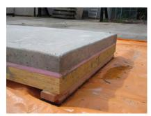
Composite floor panel used for testing Project Name: UBC Earth Sciences Building Photo credit: Equilibrium
