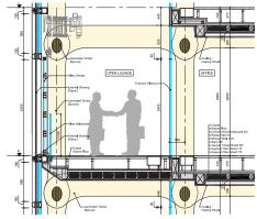
Detail of raised floor and exterior glazing Detail Credit: Shigeru Ban Architects
