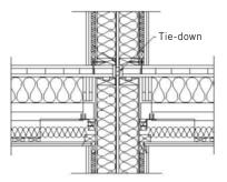
Location of tension rod through the interior wall and floor to assist with stabilization. Detail Credit: Martinsons Bryggsystem KB
