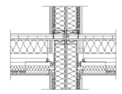
Detail showing a connection between interior wall and floor; the wall and floor elements are discontinuous at the joint. Detail Credit: Martinsons Byggsystem KB
