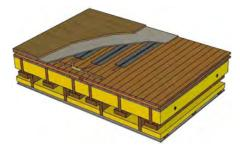
Horizontal panel showing hydronic heating channels. Detail Credit: Martinsons Byggsystem KB
