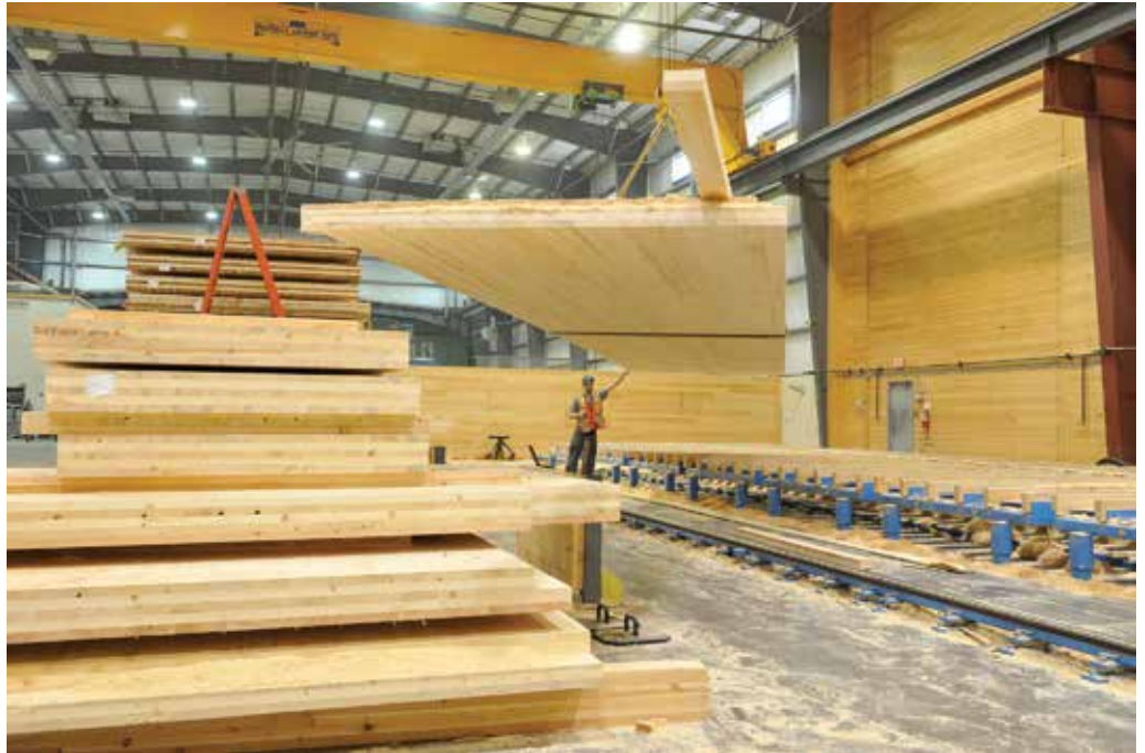
To manufacture CLT, several layers of kiln-dried lumber boards are stacked in alternating directions and bonded with structural adhesives to form solid, straight, rectangular panels.
