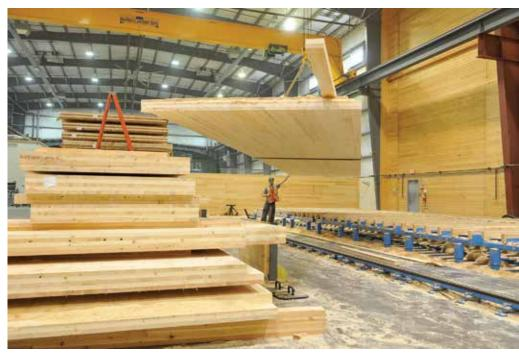
To manufacture CLT, several layers of kiln-dried lumber boards are stacked in alternating directions and bonded with structural adhesives to form solid, straight, rectangular panels.
