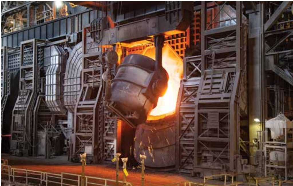
To become steel, iron must be melted and reprocessed to reduce its carbon content and remove silica, phosphorous and sulfur, which weaken the steel. Photo courtesy of Ozden Nasif, iStock by Getty Images
