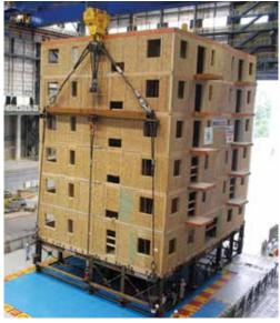
Subjected to three earthquakes on the world's largest shake table in Miki, Japan, this full-scale wood-frame apartment building performed excellently with little damage. Photo credit: John W. van de Lindt, Colorado State University
