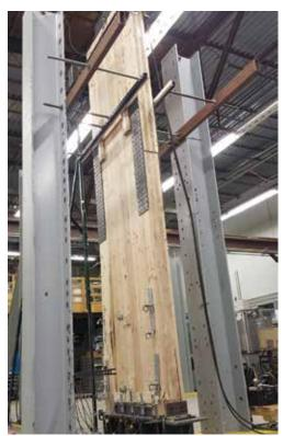
In this rocking test of a CLT shear wall, the panel maintained its lateral load-bearing strength under cycling loading to simulate seismic conditions and returned to a vertical position at completion of the test. Photo credit: ARUP
