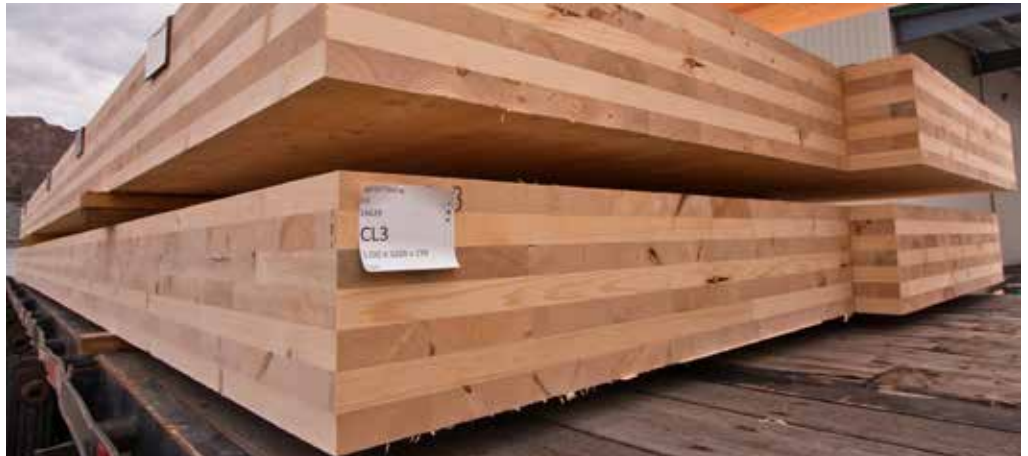
CLT is the basis of the tall wood movement, as the material's high strength, dimensional stability and rigidity allow it to be used in mid- and high-rise construction. Photo courtesy of Structurlam
