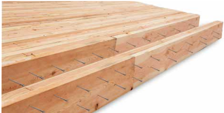
NLT gets its strength and durability from the nails that fasten individual dimension lumber, stacked on edge, into a single structural element. Photo courtesy of Think Wood
