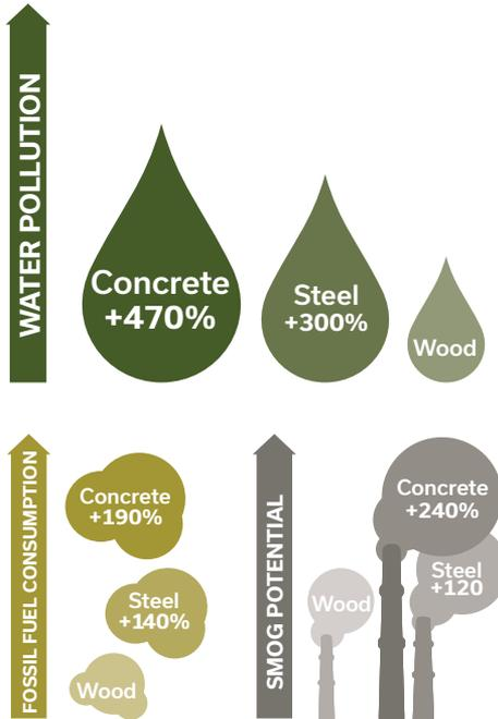
Based on a comparison of equivalent 40,000 square foot 2-story wood, steel + concrete buildings, each assumed to have a concrete foundation and slab.
