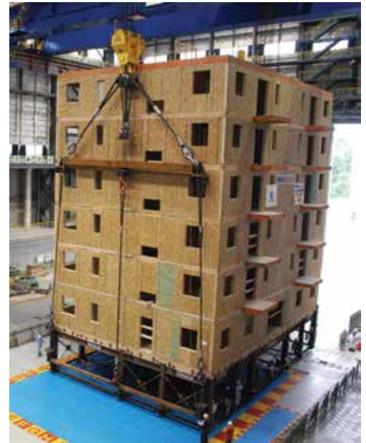
After being lifted to a shake table and subjected to four progressively intense earthquakes, this six-story light-frame building was found to have only minimal damage to the gypsum wallboard and nail connections. (View a video of the test on YouTube. 3 )
