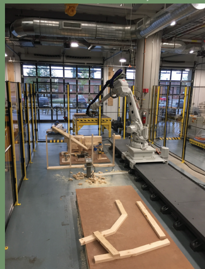
A robot at Perkins+Will's Building Technology Lab converts complex curved designs into NLT structures.
