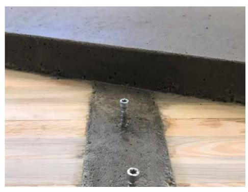
Most mass timber panels can be made into a wood-concrete composite by applying a concrete topping in such a way that the two materials act as one. Product sample courtesy of StructureCraft
