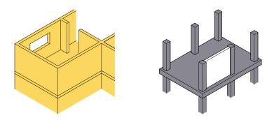
The diagrams illustrate that a CLT frame includes internal walls, as well as structure, compared to a reinforced concrete frame, which requires infill.
