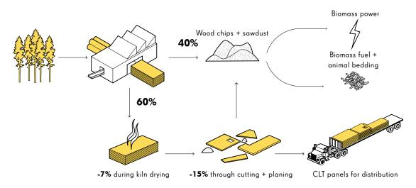
The production of CLT is a closed loop process in which most waste is reused. The diagram shows the principal activities and efficiency.
