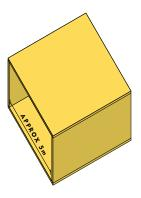
**PURE CLT** CLT forms all principal structural elements.
