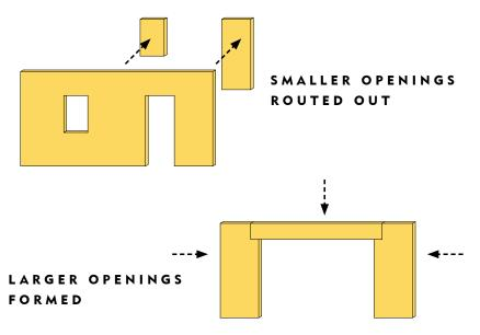
Where particularly large openings are needed it can be more cost effective to form openings from multiple pieces of CLT. The benefits should be considered against the additional lifts on site and additional joints that can increase the construction period and have the potential to reduce accuracy and structural performance.
