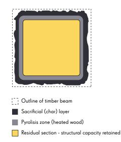
Typical spruce CLT panels char at a average rate of around ¼ inch in ten minutes (0.7mm/min), with the initial rate on each layer exceeding this temporarily.<sup>6</sup> By oversizing elements to allow for a sacrificial zone, the
