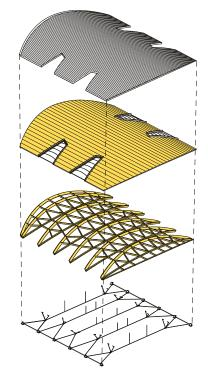
Exploded Diagram of Roof Structure
