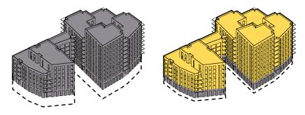
The diagram indicates an approximate reduction in the raft foundations required for a CLT version of the Dalston Works scheme.
