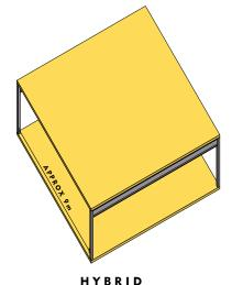
CLT slabs supported by a concrete or steel frame.
